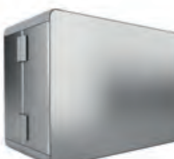
PPD 210 (Combi 150/60) The 210 mm deep enclosure consists of the combination of a 150 mm and a 60 mm basic profile. It features locks and exterior hinges.
